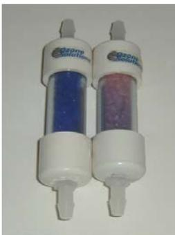
The MI-1 moisture indicator (left) will alert you to when the AD-500 requires regeneration. The indicator on the left is blue which means that the air is very dry, and suitable for ozone generation. The MI-1 on the right is purple/pink, which means that the AD-500 media must be regenerated. The MI-1 moisture indicator itself does not need to be regenerated, as it will revert to a blue color once the air having been dried by the AD-500 passes through it.
