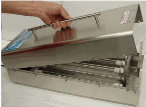
3. Clip the 4 cable ties that are holding the tubes in place.
