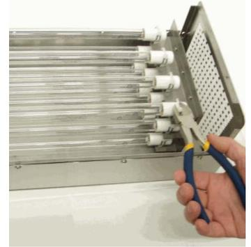
4. To remove the tube lift the end and pull while wiggling the tube back and forth being careful not to break it on the steel support / light guard.
