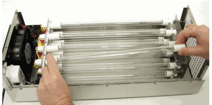
5a. To remove the lower level of tubes on the UV 2700 simply remove the ties and tubes as in step 4.
