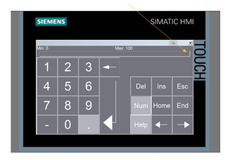
AS-500 HIGH SET POINT. THIS FIELD IS USED TO SET THE HIGH POINT ALARM. WHEN AS-500 CONTROL IS ENABLED, OZONE PRODUCTION WILL STOP WHEN IT HITS THIS SET POINT.
