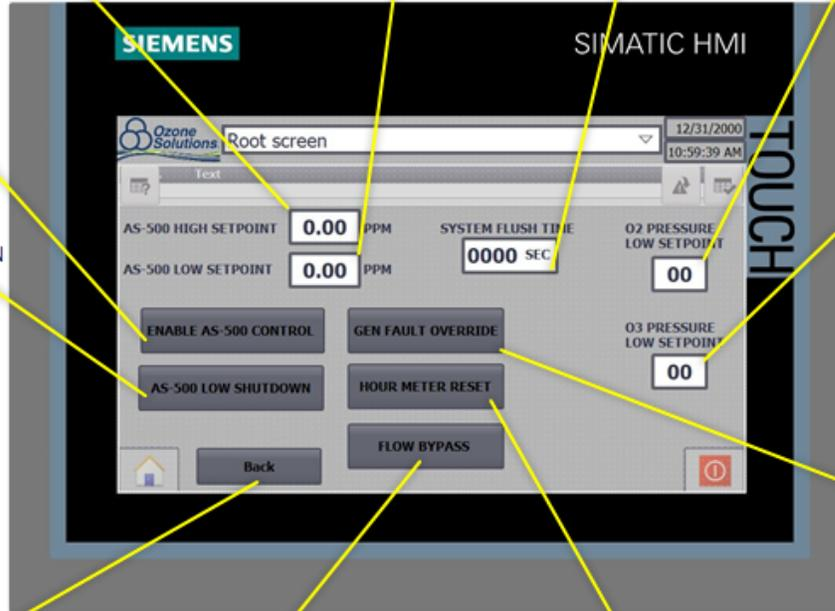
WILL BYPASS OZONE GENERATOR FAULTS. MOSTLY USED WHEN TUNING THE INVERTER BOARD (SEE INVERTER BOARD MANUAL).
