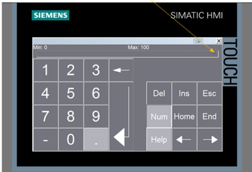
AS-500 HIGH SET POINT. THIS FIELD IS USED TO SET THE HIGH POINT ALARM. WHEN AS-500 CONTROL IS ENABLED, OZONE PRODUCTION WILL STOP WHEN IT HITS THIS SET POINT.
