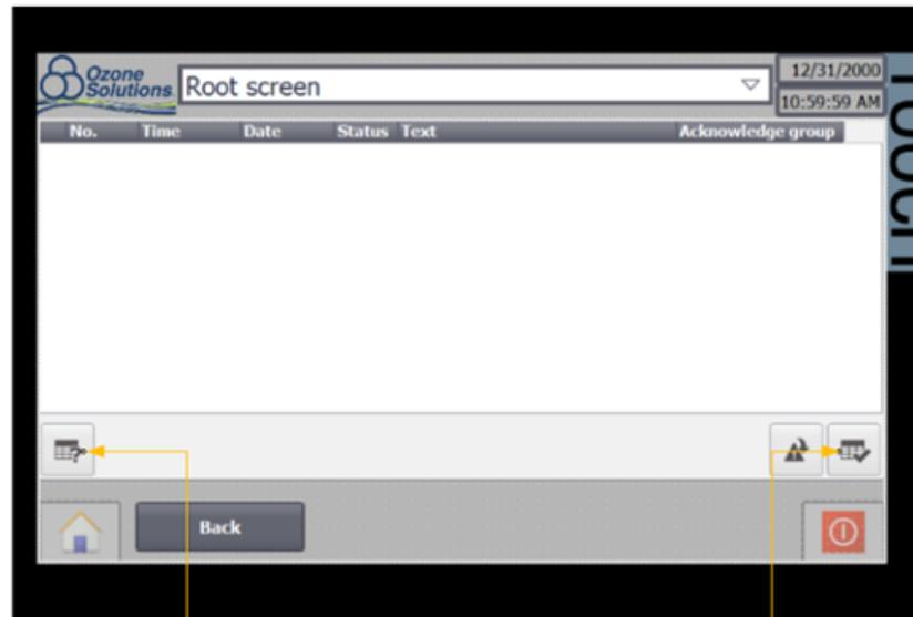
Tech tip button, when alarm is present the description of the alarm will appear when pressed
