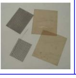
3. Take mica and stainless screens and clean in the sink using dish soap and an old toothbrush. If the plates have not been cleaned for a long time, it is important to use the tooth brush to help remove the flaking mica. Rinse with clean clear water.
