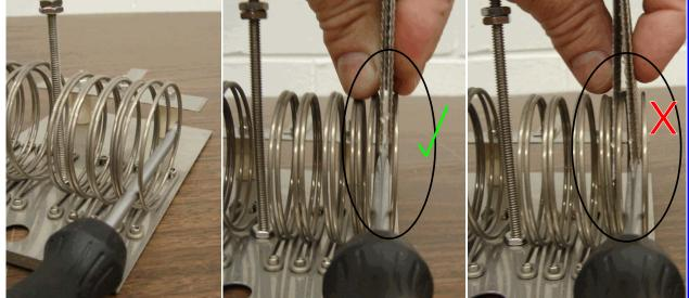
8. Re install the plate hold down bar as shown in the step 4 picture. Re install the HV clamp making sure that all the HV wires from the plates are clamped tight.
