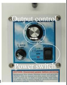
**2b.** (Setting Ozone Level (shock treatments)) For most shock treatment applications the setting should be set to the highest setting. If the area being treated is small, the setting can be reduced to a lower level.
